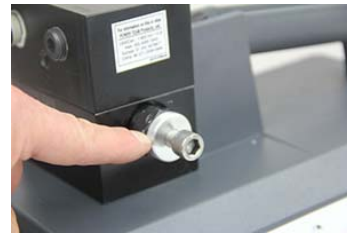
Loosen large knurled lock nut
