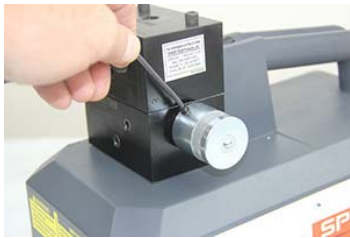
Loosen set screw on cap
