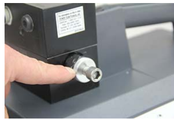
Loosen large knurled lock nut
